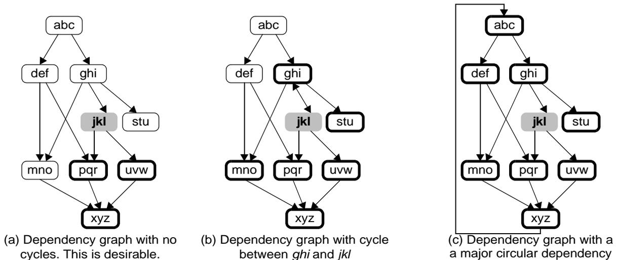
**Figure 2:** Examples of dependency graphs, without and with cycles. An objective in developing good software is to decompose code into modules to minimize or eliminate circular dependencies. In each diagram, the modules with thick borders should modules that are directly or indirectly dependent on module *jkl*, and would be needed to test or reuse *jkl*, and could be affected by any problem in *jkl*.
