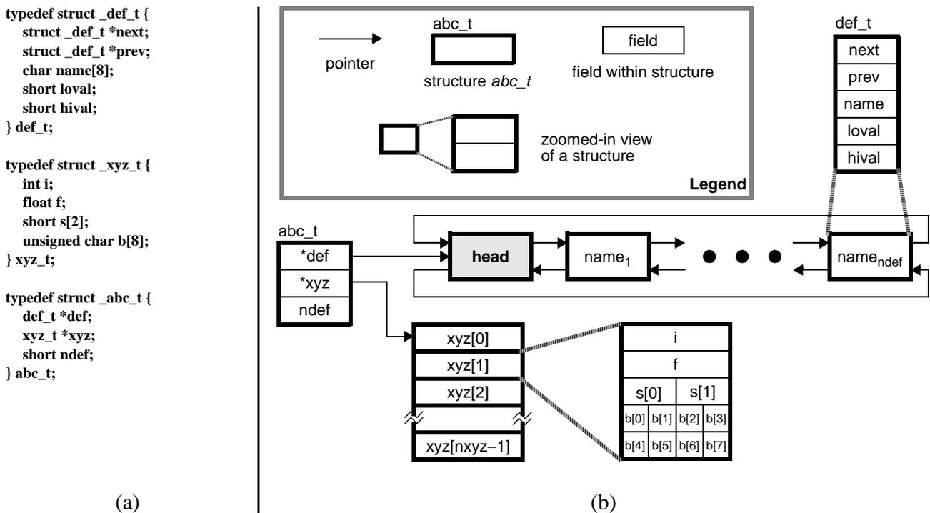
**Figure 1:** Example of a data structure diagram. Suppose that only the data structures in (a) are provided. The lack of the diagram in (b) would make it extremely difficult to understand the true structure of the design. Providing the diagram in (b) significantly improves the ability to visualize the design.
